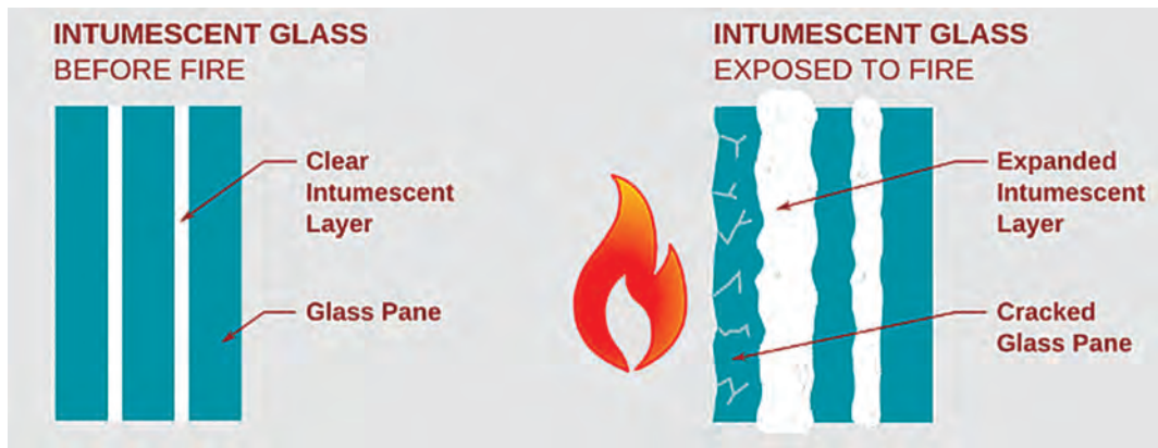
FIG. 60 INTUMESCENT-LAYER TYPE FIRE-RESISTANT GLASS
